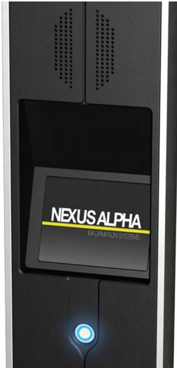
MAIA AV (shown here) is fitted with a small low power LCD display (6.5" diagonal) which is powered on demand.
