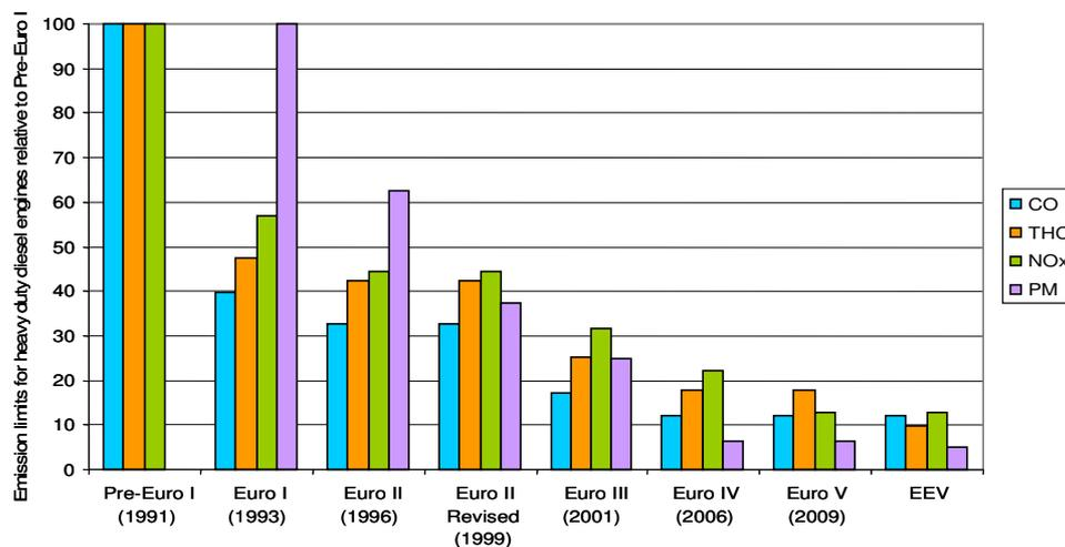
The above graph shows what has been achieved with a continuous and long term forward plan for tailpipe emissions, with the projected level of tailpipe emissions being approximately 10% of pre Euro 1 levels.
