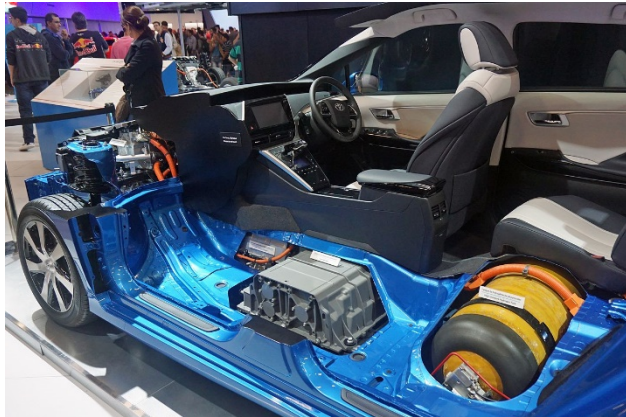
Figure 4.3 Toyota Mirai Fuel Cell Compartment
