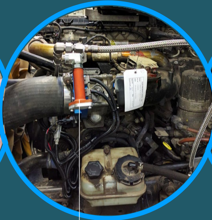
H 2 injection manifold in-line with air intake blends H 2 and air before entering engine block
