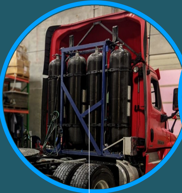
H 2 tanks & gas handling components behind or under cab
